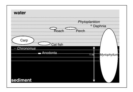
**Figure 1.** Schematic representation of the selected reference organisms and their location and ellipsoid geometries taken into account to calculate the concentration-to-dose rate coefficient for external and internal irradiation pathways.
